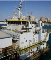
A Self-propelled Barge specifically built to provide support to offshore oilfield maintenance and construction in shallow waters.
